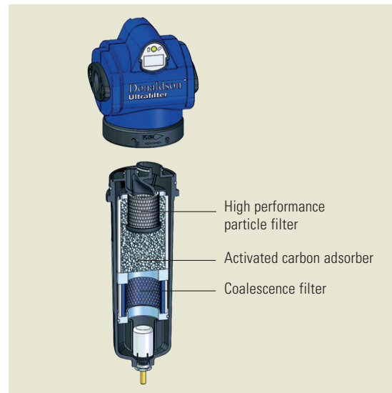
Cross-section of an Ultra-Filter with DF-T element
