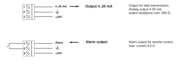
The selection of the outputs (Alarm contact or output 4-20 mA) is done via software by using the mode button and the display of the Economizer.
